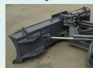
The 6-way dozer blade has Power, Angle and Tilt capability (PAT) operated from the cab. With a single control lever, the blade can be angled 25 degrees to the left or right for dispensing earth and materials away for the operator's path. The blade also tilts up on the left and right sides by 455 mm for slope grading, culverts and ditches.
