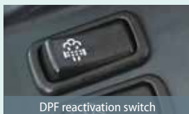
DPF reactivation switch
