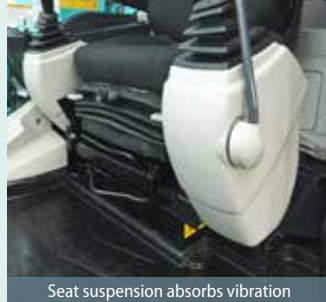
Seat suspension absorbs vibration
