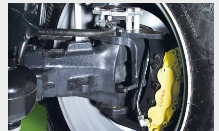
60 km/h and maximum safety with external disc brakes.
