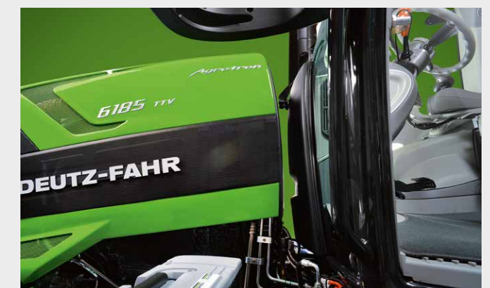
Cab and bonnet are separated to reduce noise and vibration and increase comfort.
