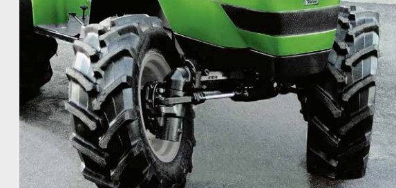
↑ With a 57 degree steering angle, the Agrokid has a very small turning radius. The portal axle provides for an exceptionally high ground clearance of up to 390 mm.
