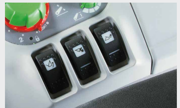
↑ ... controls for front loader operation are fully integrated and easy to reach.
