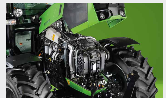
FARMotion engine with SCR exhaust gas post-treatment system. Stage III B models don't need AdBlue.
