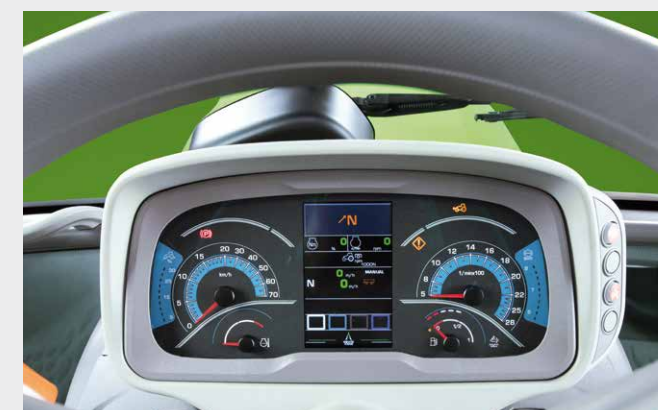
Dashboard cluster with new InfoCentrePro: 5" high-res LCD color display for customisable top information concept.
