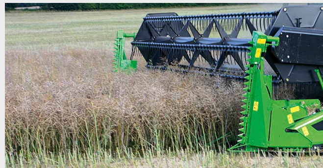
For rape harvesting there is a specifically designed kit which can be applied to the standard DEUTZ-FAHR headers up to 7.2 m.
