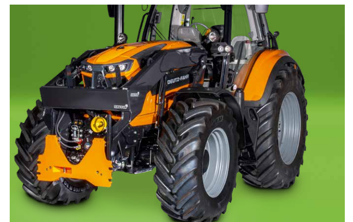
Support frame from Sauter with adjustable communal pallet (category 3/5) and axle support for heavy attachment loads and outrigger.
