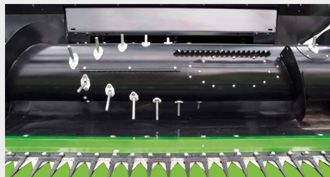
Large diameter of the intake auger with adjustable fingers in spiral all along the entire cutting width.
