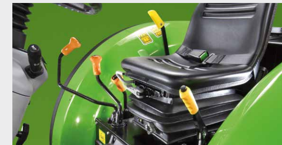
↑ The operator driving position is logical and comfortable, and the gear levers are located on the right-hand side of the seat so that the operator can get on and off the platform unimpeded.
