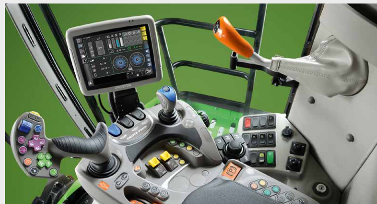
↑ With the new armrest integrating the COMMANDER STICK and the iMonitor you can perform all combine harvester adjustments in a simple and effortless manner.
