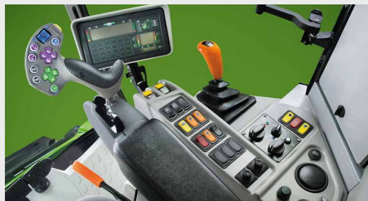
Modern cab with new console and adjustable, three-position steering column.
