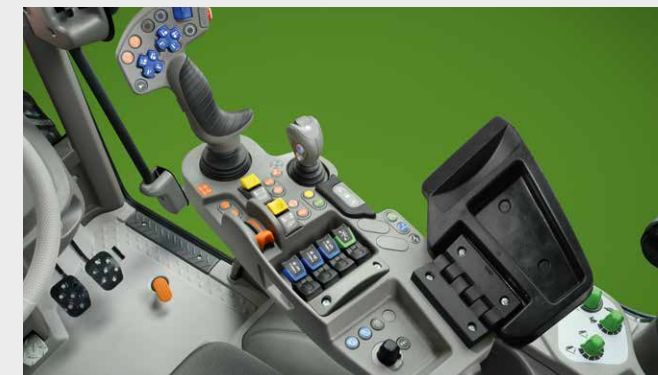
↑ The MaxCom armrest with ergonomical joystick and clearly colour coded functions.
