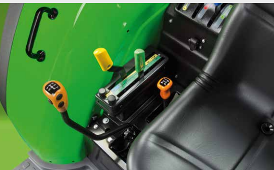
↑ Transmission, rear lift and spool valves mechanical controls.
