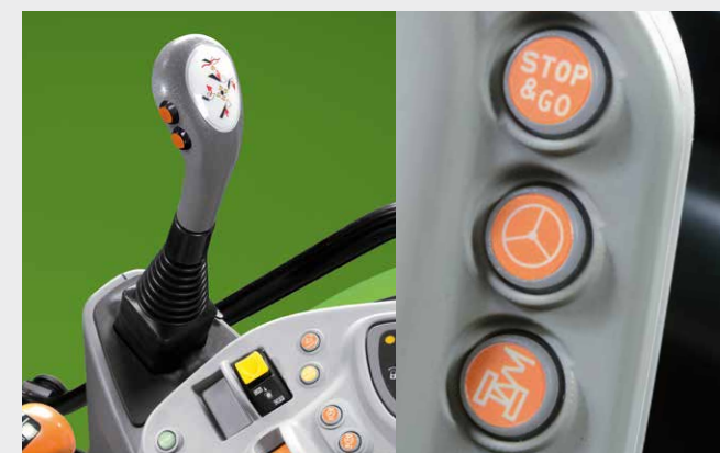
↑ Depending on the tractor model, front loader joystick with Powershift buttons. Stop&Go, SDD rapid steering system and all...
