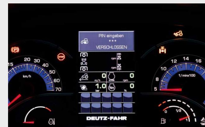
State of the art dashboard with InfoCentrePro: 5" colour display and high resolution for a user-defined information concept at top level. Security thanks to code lock. Lock and unlock with PIN.
