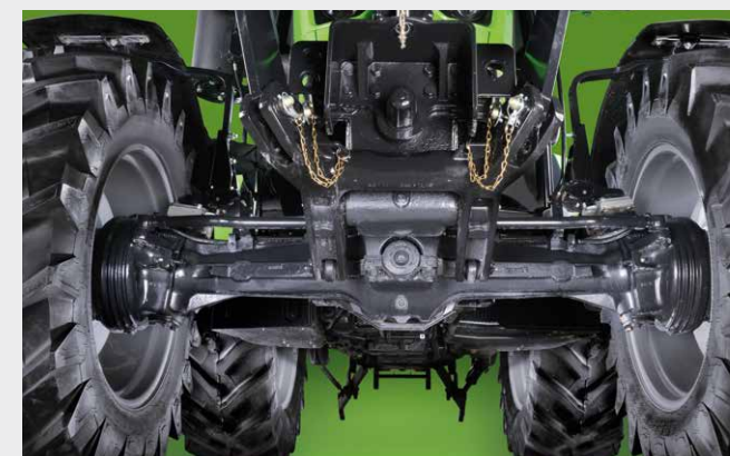
↑ The front axle features a new suspension for more driving comfort, safety and grip.
