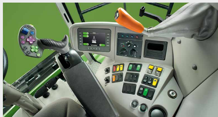
Easy access to all controls, multifunctional COMMANDER Stick and 7" touch screen display always visible in all conditions.
