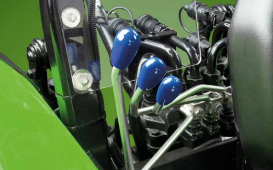
↑ Fitted with up to 3 mechanical control valves.
