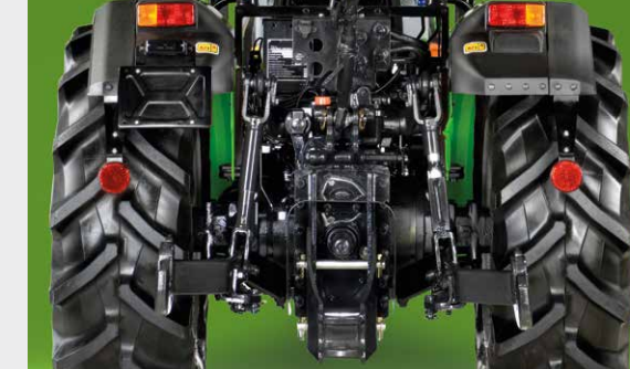
↑ 3-speed PTO (540 / 540ECO / 1000) and ground speed PTO for all kinds of applications.
