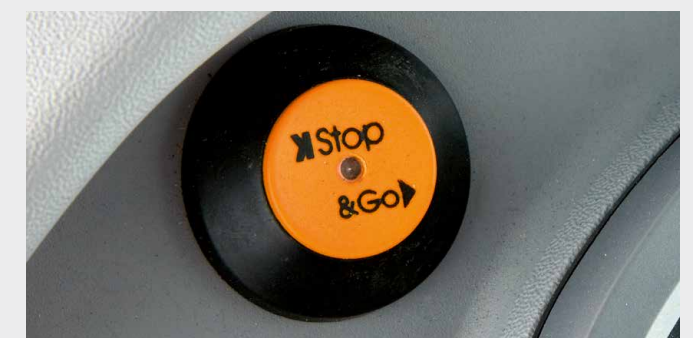
With Stop&Go, you can control the tractor's movement by only using the brake pedals, without even touching the clutch pedal.
