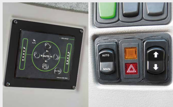
↑ Independent control between front BALANCE and rear levelling system, both with automatic or manual function.
