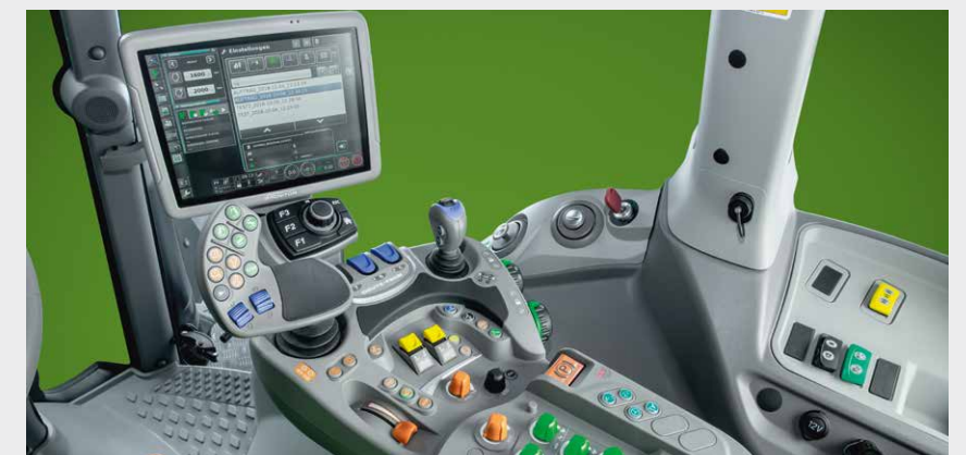
The multifunction armrest of the 7 Series TTV incorporates all the main controls and allows total management of the machine.
