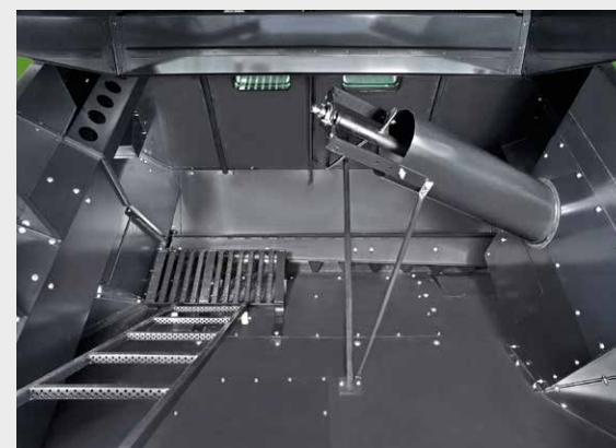
7000-litre grain tank to minimize unloading stops.
