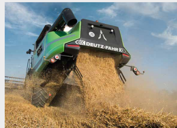
↑ The new C9300 Series offers a new design of the straw-hood to improve the efficiency with long straw and increase the effectiveness of the straw-chopper.
