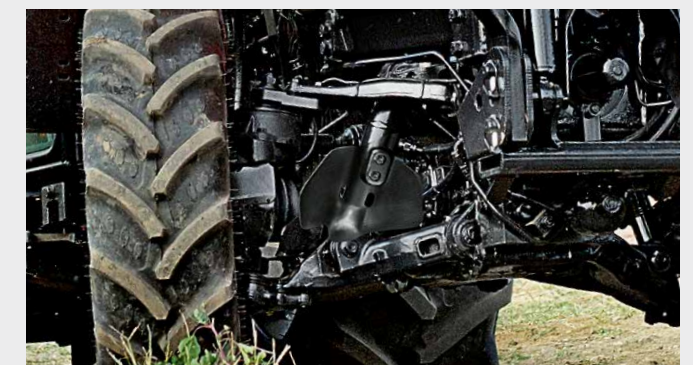
Independent wheel suspension with double wishbone design.
