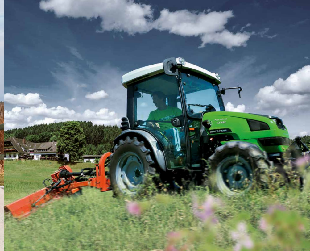
↑ With a 57 degree steering angle, the Agrokid has a very small turning radius. The portal axle provides for an exceptionally high ground clearance of up to 390 mm.
