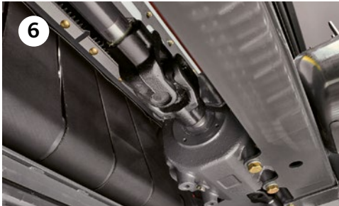
Heavy duty cross joints in the drive axles
