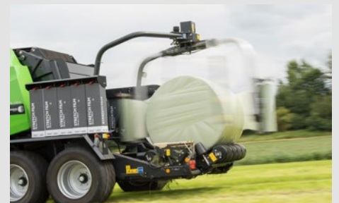
Switches to conventional wrapping for 100% film coverage.
