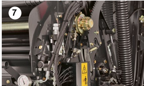
Proportional valve for in-cab density control
