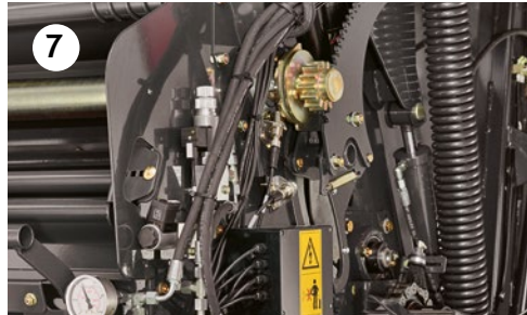
Proportional valve for in-cab density control
