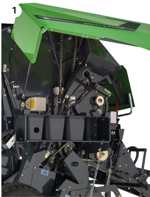
Robust driveline with high quality IWIS chains
