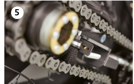
5 Sturdy and wide oil brushes on the chains ensure perfect lubrication
