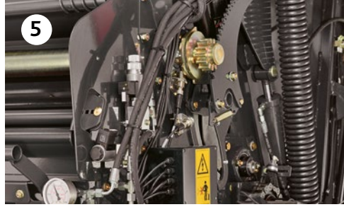
Proportional valve for in-cab density control
