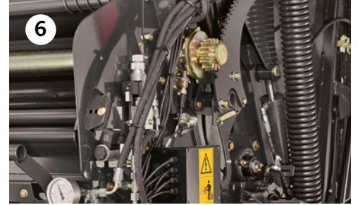
Proportional valve for in-cab density control
