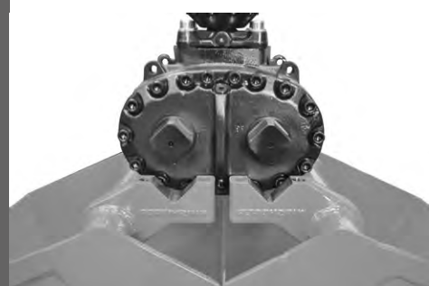
Lift HPXdrive for exchange of shells
