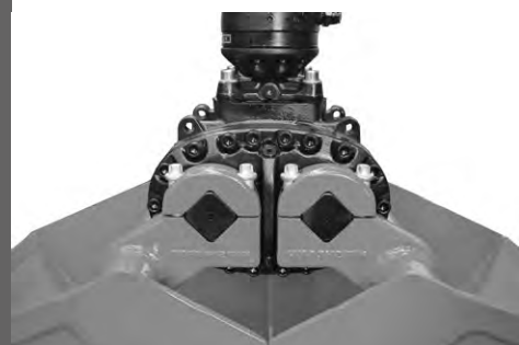
Loosen 4 bolts on each side
