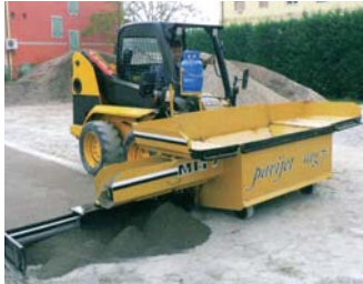
Stende asfalti, cemento, sabbia e inerti Lays asphalt/macadam concrete job base
